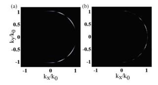
FIG. 4. (a) Simulated Fourier plane of a coherent source placed at 850 nm from a mirror with a reflection coefficient r = 1. (b) Fourier plane acquired for a fluorescent nanobead placed at 850 nm from a SPP Bragg mirror.
