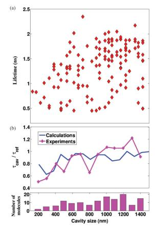
FIG. 11. (Color online) (a) Fluorescence lifetime as a function of the cavity size. (b) Average lifetime as a function of the cavity size (purple curve). The blue curve is calculated assuming a mean molecule position z = 25 nm above the metal film. Lifetimes are normalized with respect to the reference measured ( $\tau_{ref} = 1.43$  ns) or calculated ( $\tau_{ref}/\tau_0 = 0.51$ ) far from the cavity. The bottom panel depicts the number of considered molecules for each cavity size.
