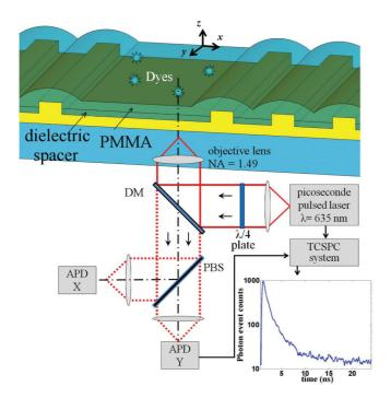
FIG. 8. (Color online) Confocal FLIM setup. Dye molecules randomly deposited into a plasmonic cavity are excited with a circularly polarized laser beam. Fluorescence emission is divided by a polarized beam splitter (PBS) and collected on two APDs (Excelitas Technologies SPCM-AQRH-15). APD-Y is connected to a timecorrelated single photon counting card (TCSPC; Picoquant-PicoHarp 300) for fluorescence decay acquisition (inset).
