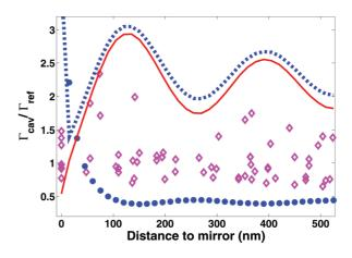
FIG. 13. (Color online) Measured normalized decay rates as a function of distance to the closest mirror for a cavity length  $L_{cav} = 1.1 \ \mu m$  (purple diamonds). Decay rates calculated for a *z*-oriented (dashed curve) and an *x*-oriented (dots) dipole are also shown. The calculated radiative decay is plotted for a *z*-oriented emitter (solid red curve).
