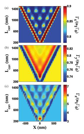
FIG. 10. (Color online) (a), (c) Normalized fluorescence decay rate as a function of cavity size  $L_{cav}$  and molecule position for x-(a), y- (b), and z- (c) oriented emitter. Decay rates are normalized with respect to their value  $n_1\Gamma_0$  in a homogeneous background of optical index  $n_1$ . The value outside the cavity refers to the decay rate in absence of the gold gratings.
