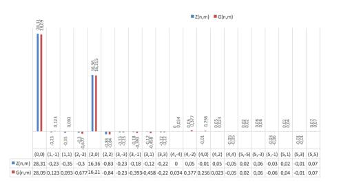
FIGURE 8. A high myopia. Wavefront decomposition in the Zernike and the  $LD - HV_2$  basis.
