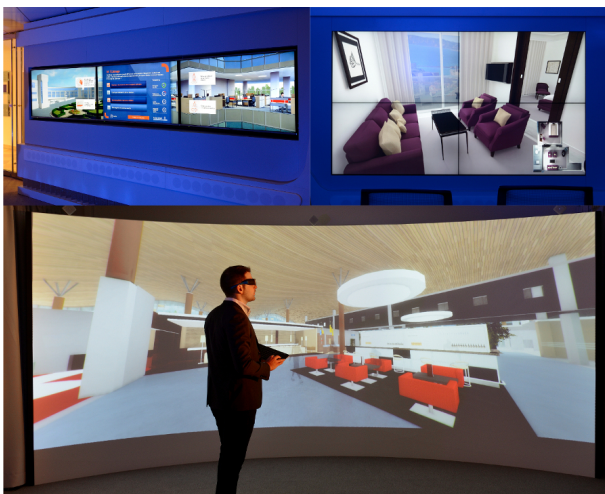
Figure 3. Pictures of the systems from the Arcas room. Top-left: the 3 TV system for additional displays. Top-right: the wall of screens. Bottom: cave system.
