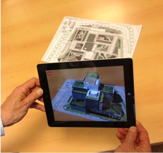
Figure 4. Augmented applications for the construction. The tablet captures the printed plan and superpose the 3D model of the corresponding project on it.
