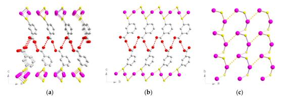
**Figure 2.** Structure representations of  $[Au(m-SPhCO_2H)]_n$ . Views of **(a)** (ac) and **(b)** (bc) planes. **(c)** View of the Au–S chains on the (ab) plane. Pink, Au; yellow, S; red, O; grey, C. Hydrogen atoms are omitted for clarity. Red and orange dotted lines represent the hydrogen bonds and interchain aurophilic interactions, respectively.
