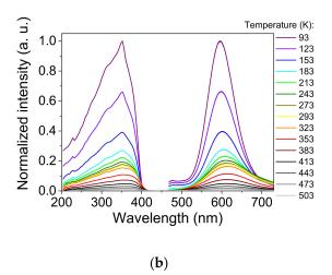
**Figure 3.** Luminescent properties of  $[Au(m-SPhCO_2H)]_n$ : (a) 2D map of the emission and excitation spectra conducted in a solid state at room temperature; (b) emission and excitation spectra ( $\lambda_{exc} = 352$  nm,  $\lambda_{em} = 596$  nm) in a solid state at varying temperatures.
