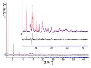
**Figure 1.** Final Rietveld plot of [Au(*m*-SPhCO<sub>2</sub>H)]<sub>n</sub> showing observed (blue circles), calculated (red line), and difference (black line) curves. Zoomed-in high angles are shown as an inset.
