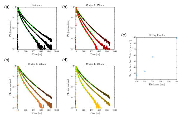
**Figure S3**: Fitting result of the time resolved measurement. (a-d) Experimental decays at three fluences (4, 10, 30e11 ph.cm<sup>-2</sup>) overlaid with the fitting model (green dashes). (e) Fitted top surface recombination velocity as a function of the thickness of the Ar etched crater.
