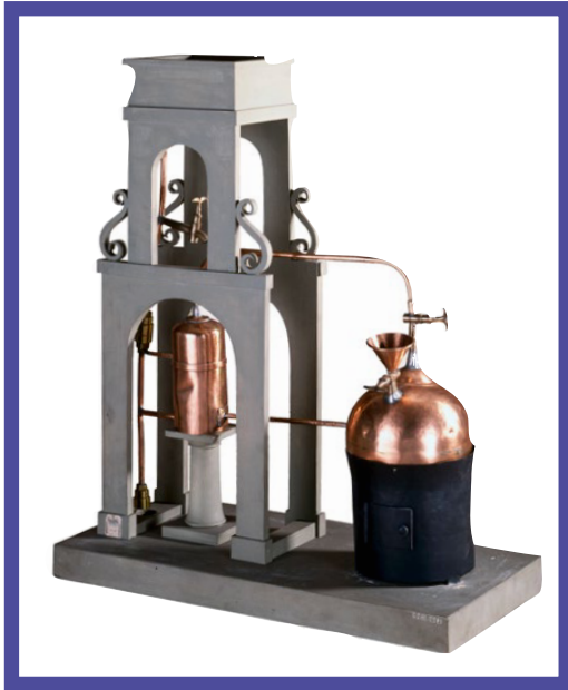
Pioneer Steam engine by Savery, model of 1753. This first steam engine received a patent in 1698. Dangerous and inefficient, it was only used to supply the fountains of princely gardens.
