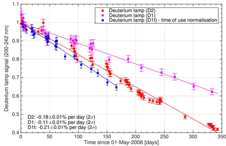
**Figure 1.** Temporal variations of SOLAR/SOLSPEC signal (200–242 nm) during calibrations with deuterium lamps (D1 and D2). The blue curve (D1t) represents the normalized temporal variation during a calibration with the D1 lamp for the same operation time as the D2 lamp.
