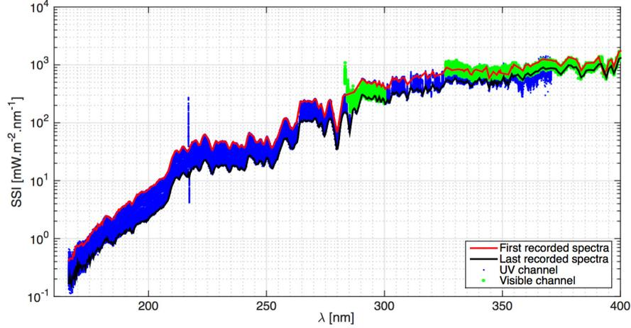
**Figure 2.** Measured spectral distribution of UV SSI (165–400 nm) from April 2008 to August 2015. Measurements of the ‘UV’ spectral band are represented with the blue dots. Measurements of the ‘VIS’ spectral band are represented with the green dots. The red curve represents the first SOLAR/SOLSPEC UV spectrum. The black curve represents the last UV solar spectrum obtained in August 2015.
