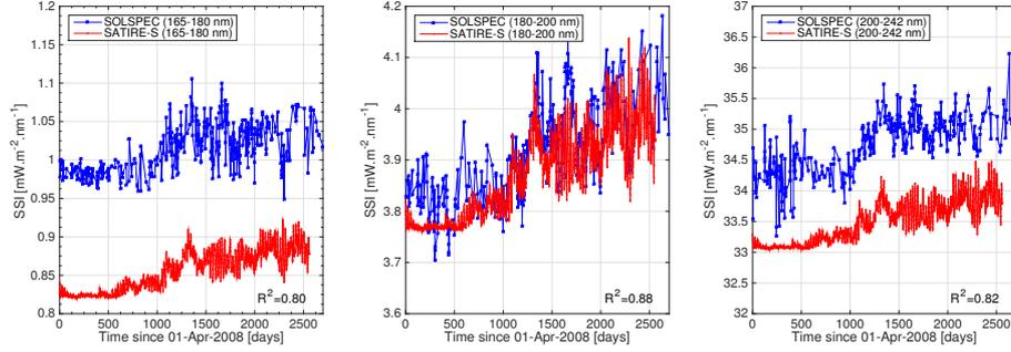
**Figure 11.** UV SSI variability in three spectral bands (165–180, 180–200, and 200–242 nm) during Solar Cycle 24. The blue curves with dots correspond to the measurement made by SOLAR/SOLSPEC. The red curves represent the values obtained with the SATIRE-S model.  $R^2$  is the Pearson’s linear correlation coefficient between SOLAR/SOLSPEC and SATIRE-S data.
