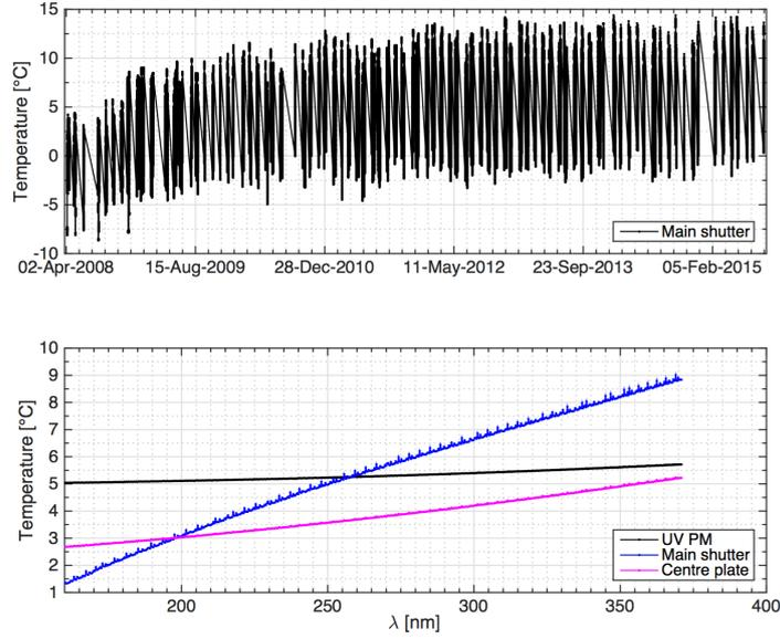
**Figure 5.** (top) Temperature evolution of SOLAR/SOLSPEC main shutter from April 2008 to mid-2015. (bottom) The Y-axis represents the mean temperatures (UV PM, main shutter, and SOLAR/SOLSPEC centre plate) from April 2008 to mid-2015 during SSI measurement with the ‘UV’ spectrometer at a given wavelength (X-axis).
