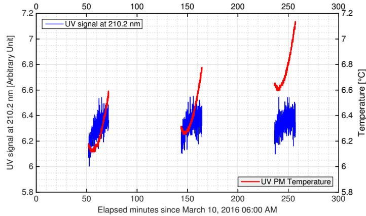
**Figure 3.** The red curve represents the UV PM temperature evolution during a calibration test. The SOLAR/SOLSPEC signal ( $S_n(t)$  at 210.2 nm) evolves during a short time period (the blue curve). This instability effect should be corrected.
